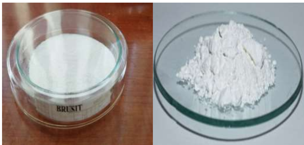
Figure 1. Magnesium hydroxide samples isolated in laboratory conditions from Dehqanabad dolomite
