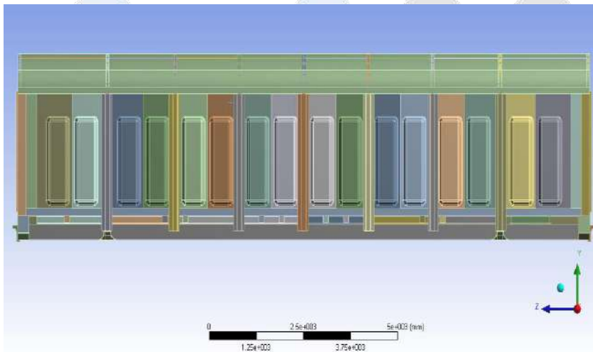
Figure 2 – Longitudinal view of the calculation model of the weighing wagon body
