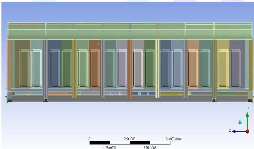
Figure 2 – Longitudinal view of the calculation model of the weighing wagon body
