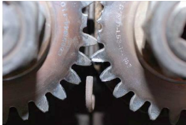
Figure 3. Damage on gear teeth caused by insufficient lubrication
