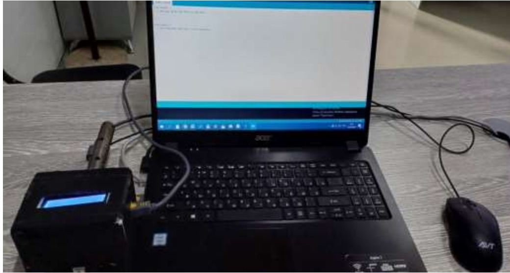
Fig. 2. Device for measuring the tension of warps.
