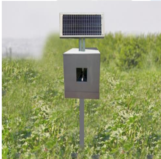
Figure 1. Insect pest collection device
