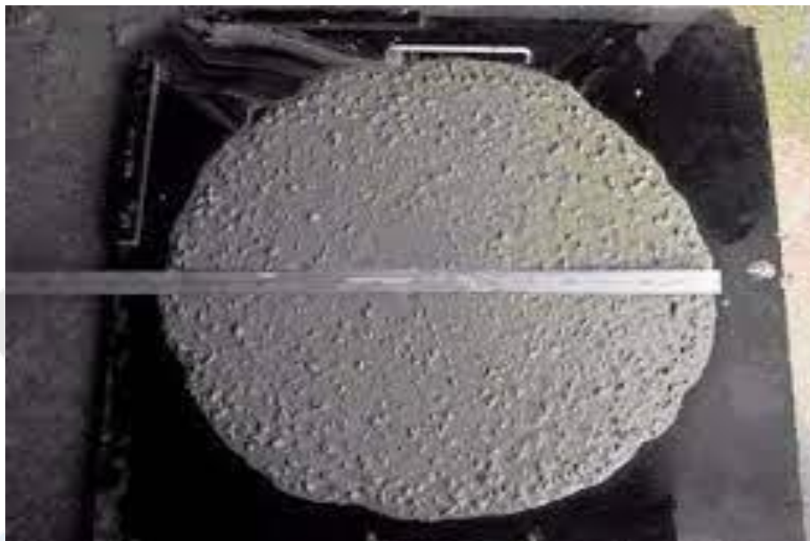
Figure 1. Spreading of concrete with superplasticizer
