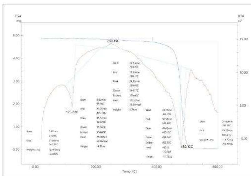
**Figure 3.19. Derivatogram of polyethylene with 3% organic pigment K-1**
