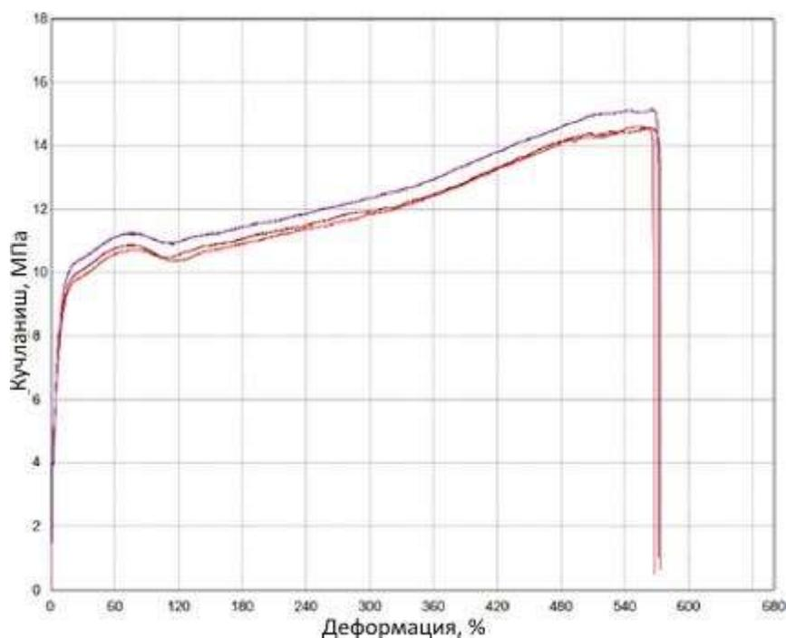
**Figure 3.14. Tensile strength diagram of K-1 grade organic pigmented polyethylene**
