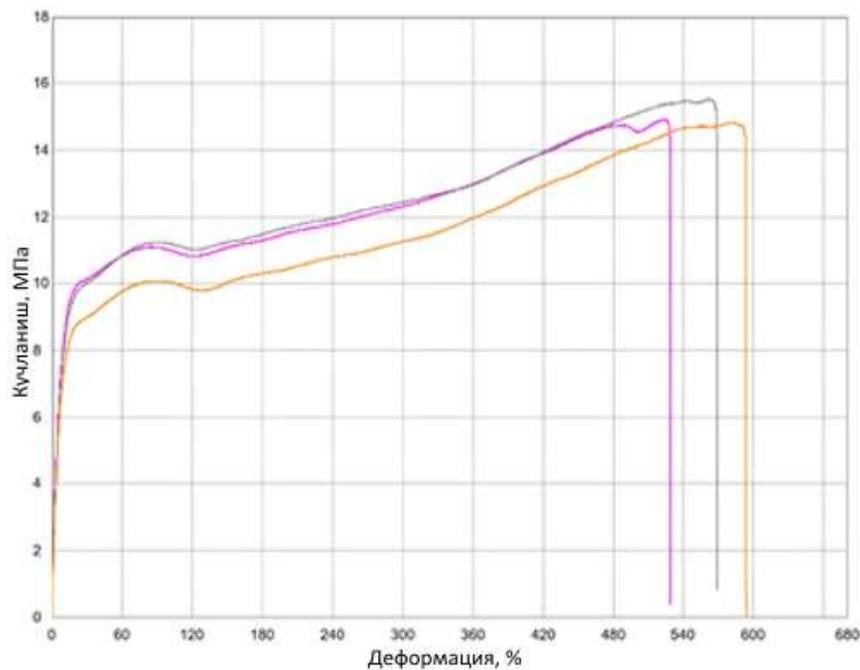
**Figure 3.16. Tensile strength diagram of polyethylene without organic pigment addition**
