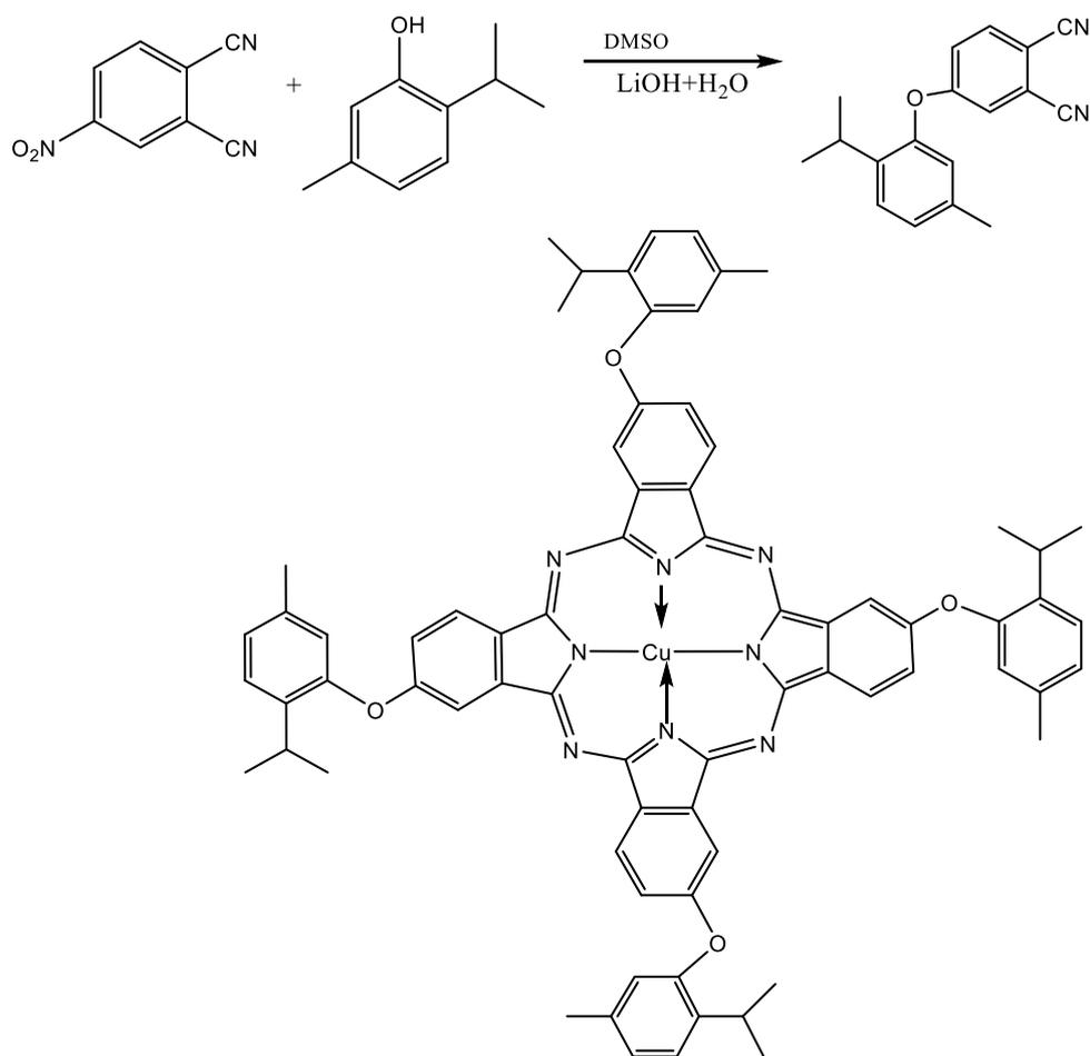
**Figure 1.2. Synthesis of copper tetra(2-isopropyl-5-methylphenoxy) phthalocyanine.**
