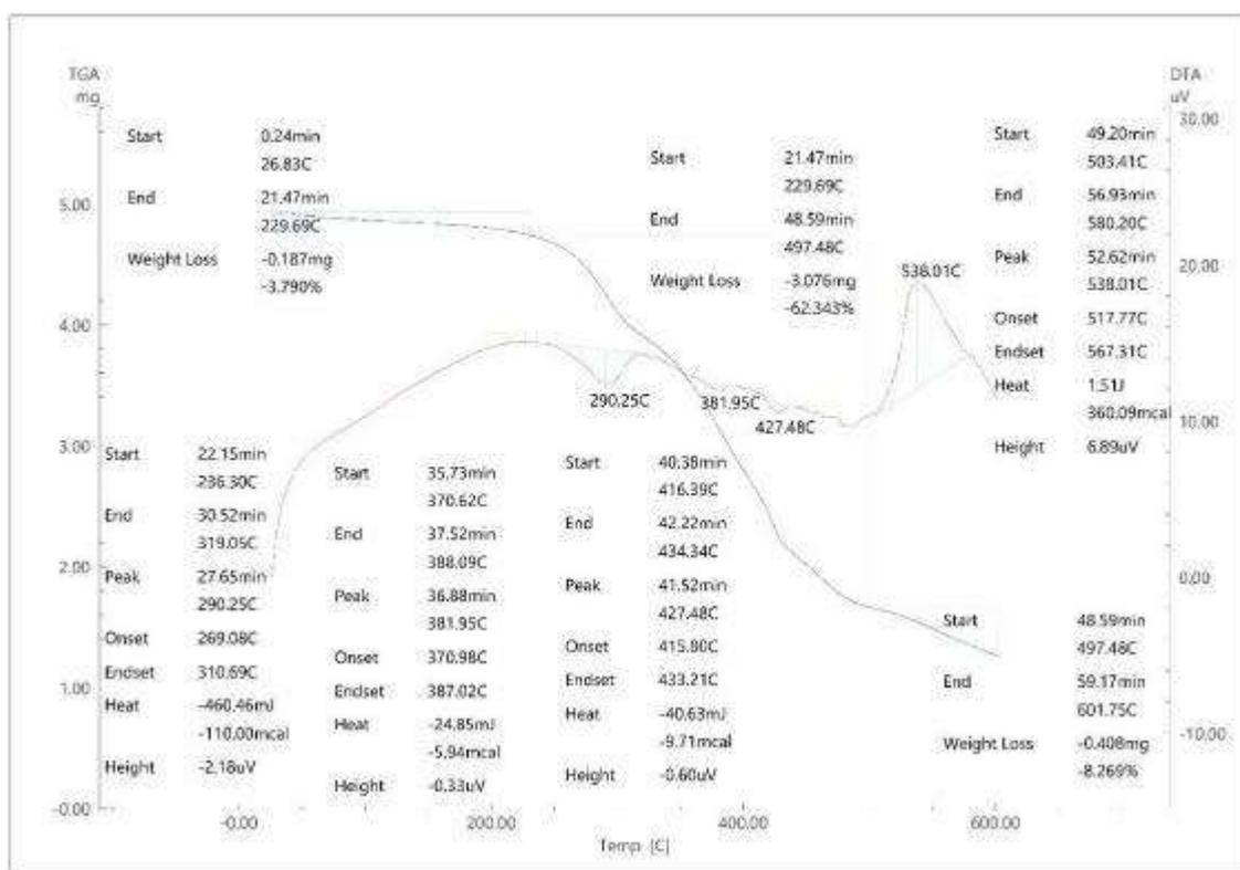
**Figure 3.2. Derivatogram of alkyd enamel made on the basis of M-1 organic pigment**
