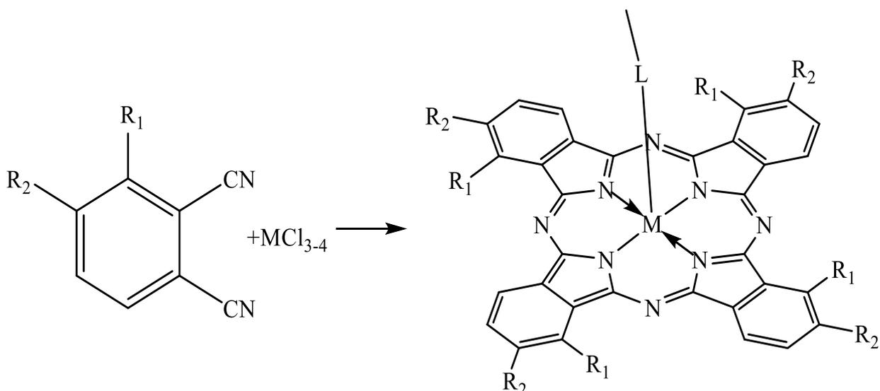
**Fig. 1.5 Preparation of extracomplexes using (III) valent metals.**
