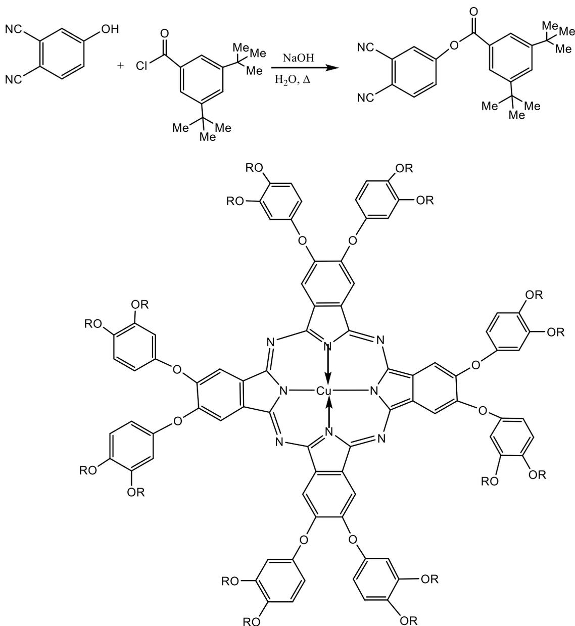
**Figure 1.3. Synthesis of phthalocyanines with phenoxy derivatives.**
