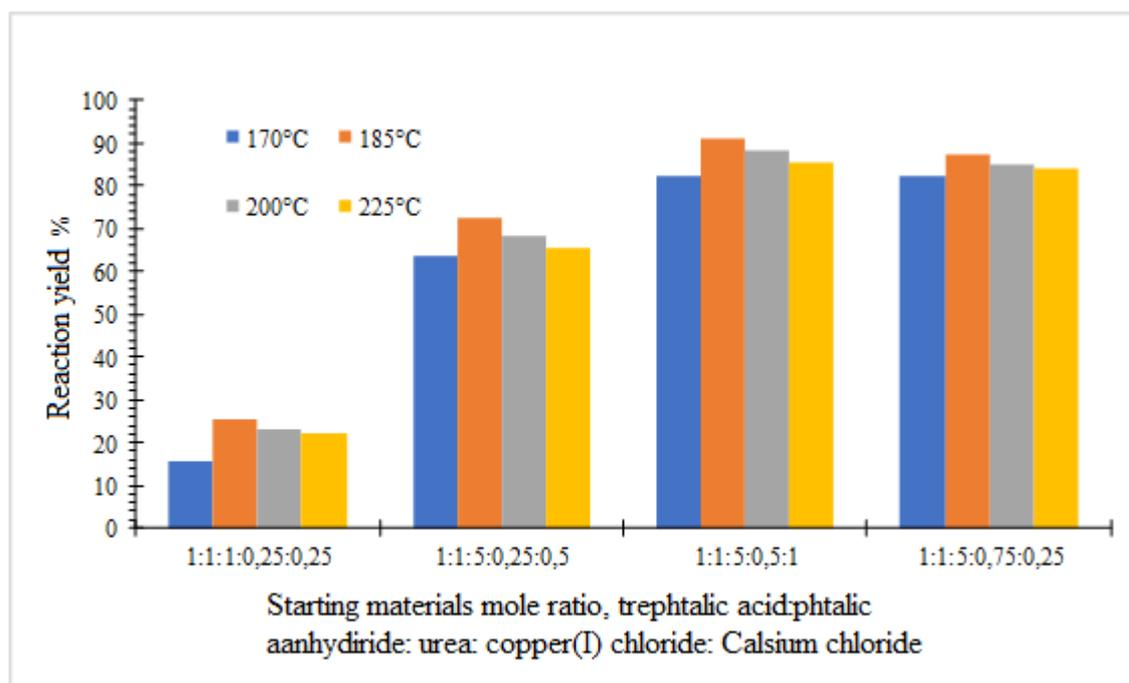
**Figure 2.2. The effect of the amount of starting materials and temperature on the reaction yield of M-2 organic pigment**
