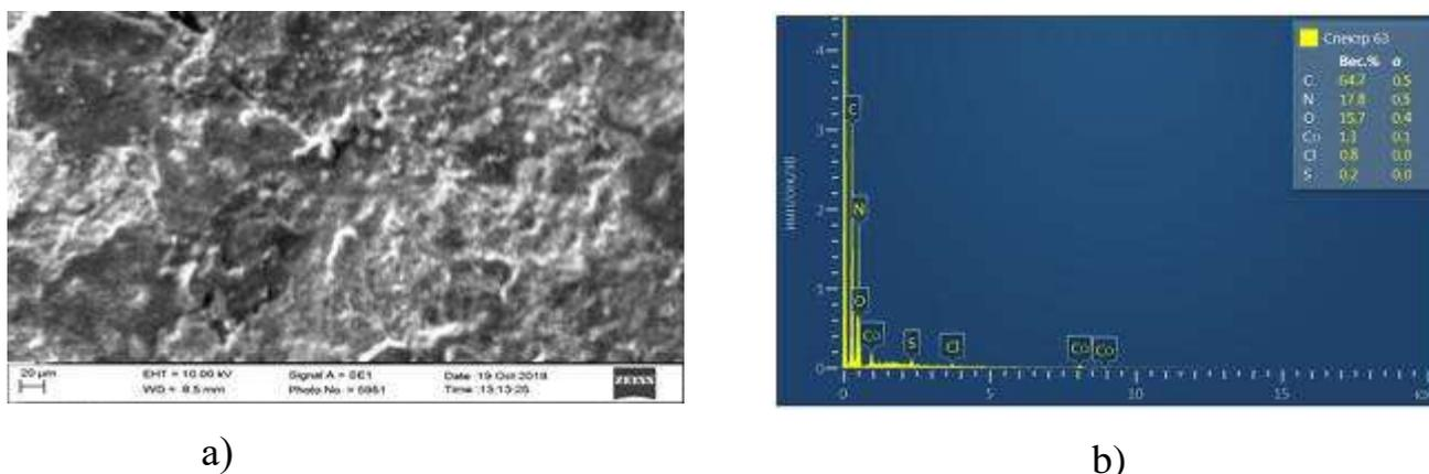
**Figure 2.27. Scanning electron microscope (a) and elemental analysis (b) data of synthesized K-1 organic pigment**
