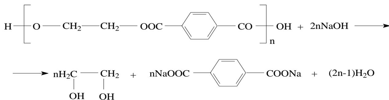
1750-1800 rpm to obtain terephthalic acid from secondary PET. A reactor equipped with a high-speed mechanical stirrer and a thermometer was used. Hydrolysis of polyethylene terephthalate is carried out in the following sequence.
