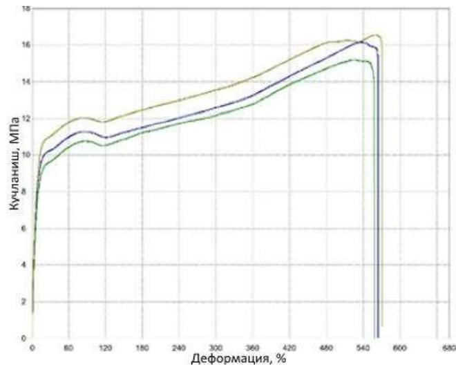
**Figure 3.15. Tensile strength diagram of K-2 grade organic pigmented polyethylene**
