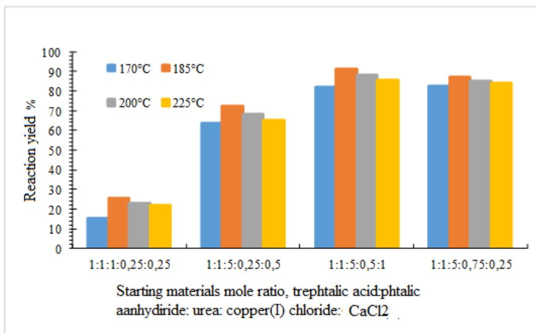
**Figure 2.4. Diagram of the effect of the amount of starting materials and temperature on the reaction yield of K-2 organic pigment**
