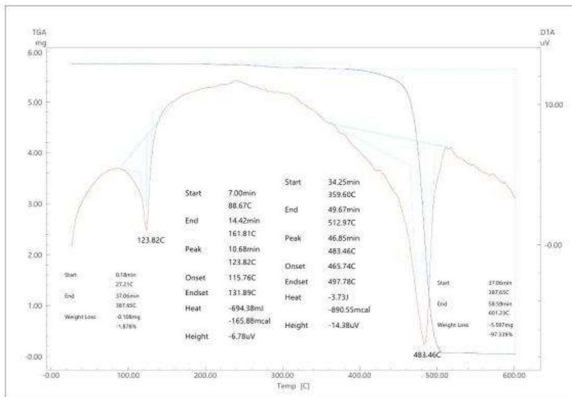
**Figure 3.17. Derivatogram of polyethylene with 3% organic pigment M-1.**
