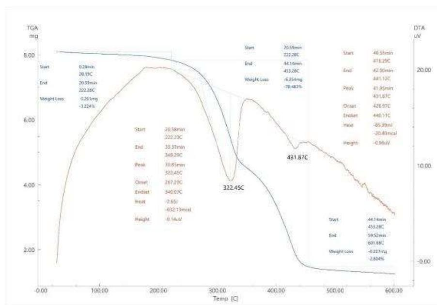
**Figure 3.5. Derivatogram of alkyd enamel made on the basis of K-2 organic pigment**
