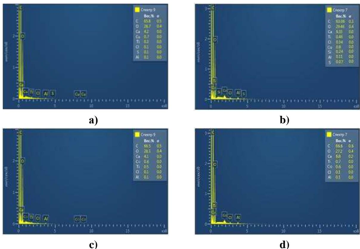
**Figure 3.7. Results of elemental analysis of paints based on new organic pigments a) M-1, b) M-2, c) K-1, d) K-2**
