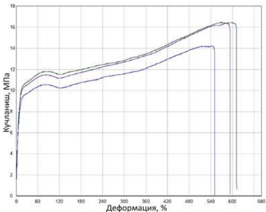
**Figure 3.12. Tensile strength diagram of M-1 organic pigmented polyethylene**
