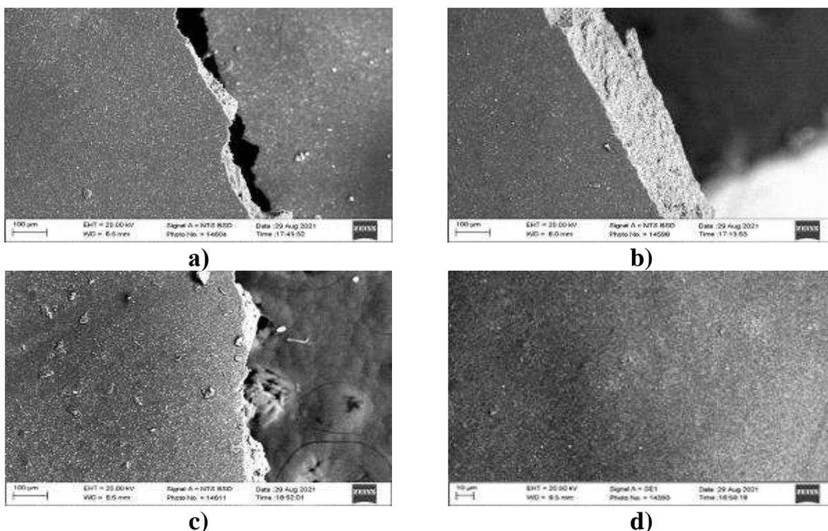
**Figure 3.7. SEM images of paints based on new organic pigments. a) M-1, b) M-2, c) K-1, d) K-2**
