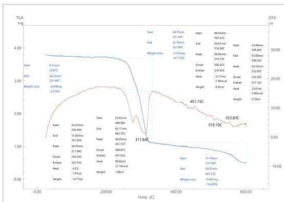
**Figure 2.18. Thermogravimetric (TG) and differential thermal analysis (DTA) derivative diagram of M-2 organic pigment.**
