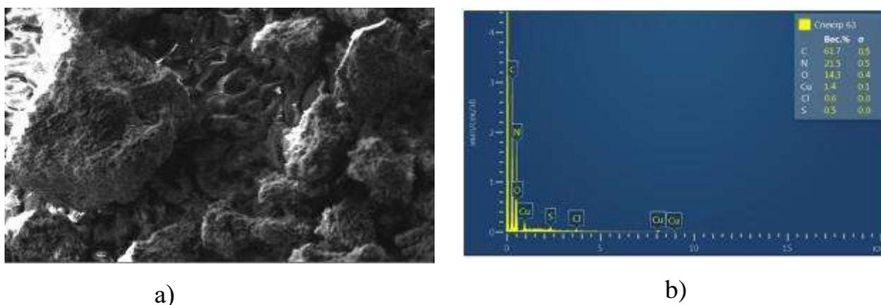
**Figure 2.25. Scanning electron microscopy (a) and elemental analysis (b) data of M-1 organic pigment**
