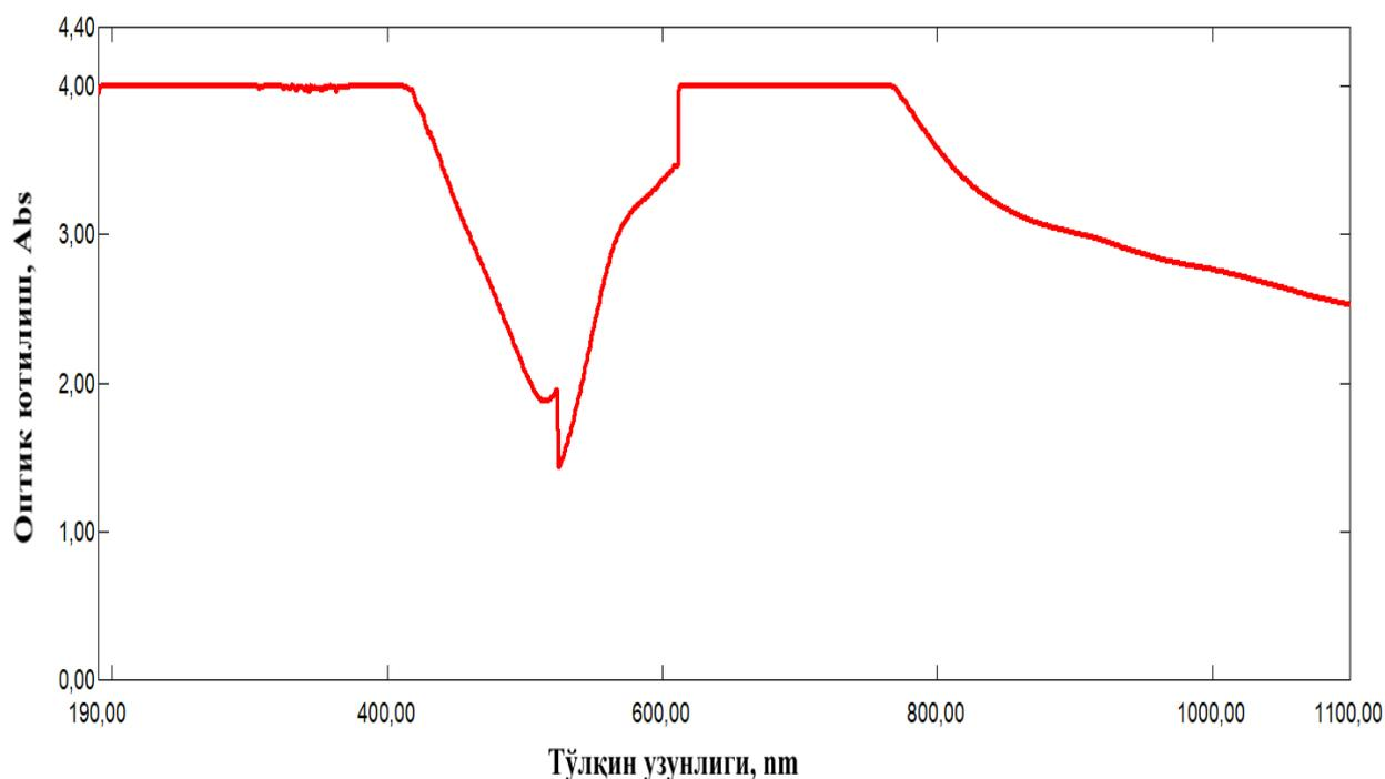
**Figure 2.13. Ratio of light absorption to wavelength of M-2 brand organic pigment**
