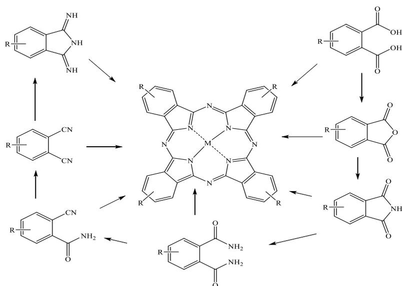
**Figure 1.1. The main substances used in the production of phthalocyanines [4].**
