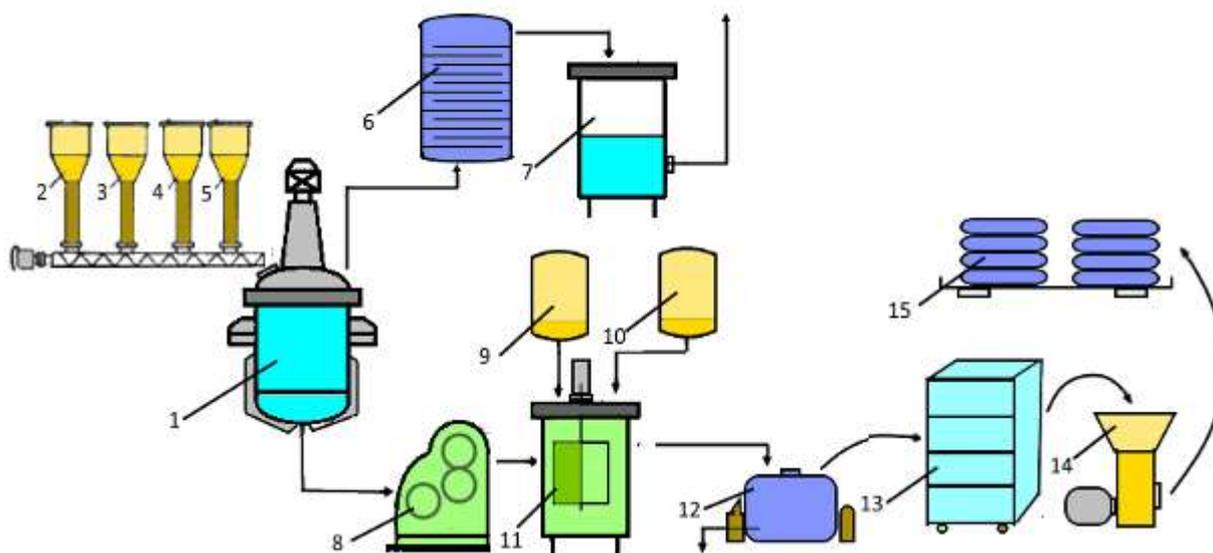
**Figure 4.1. Principle technological scheme of organic pigment production**
