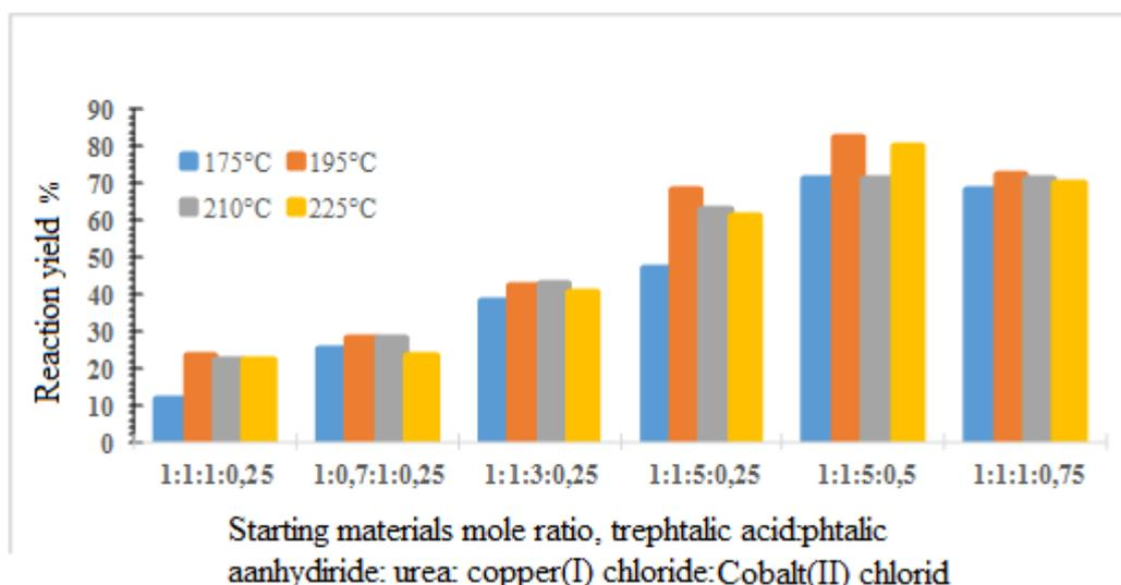
**Figure 2.3. The effect of the amount of starting materials and temperature on the reaction yield of K-1 organic pigment**
