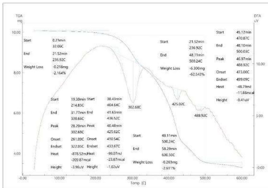
**Figure 3.3. Derivatogram of alkyd enamel made on the basis of M-2 organic pigment**
