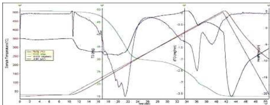
Figure 3.6 shows the derivatogram of the alkyd enamel prepared by adding the CuPc pigment taken for control.
