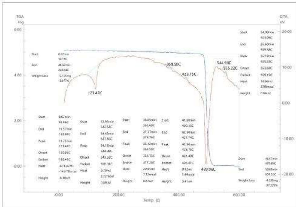
**Figure 3.18. Derivatogram of polyethylene with 3% M-2 organic pigment added**
