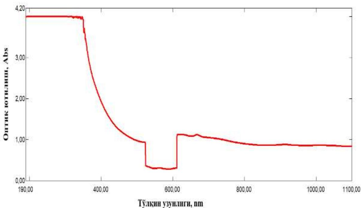
**Figure 2.12. Ratio of light absorption to wavelength of M-1 brand organic pigment**
