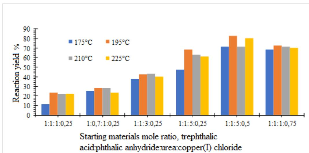
**Figure 2.1. The effect of the amount of starting materials and temperature on the reaction yield of M-1 organic pigment**
