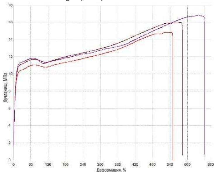
**Figure 3.13. Tensile strength diagram of M-2 organic pigmented polyethylene**
