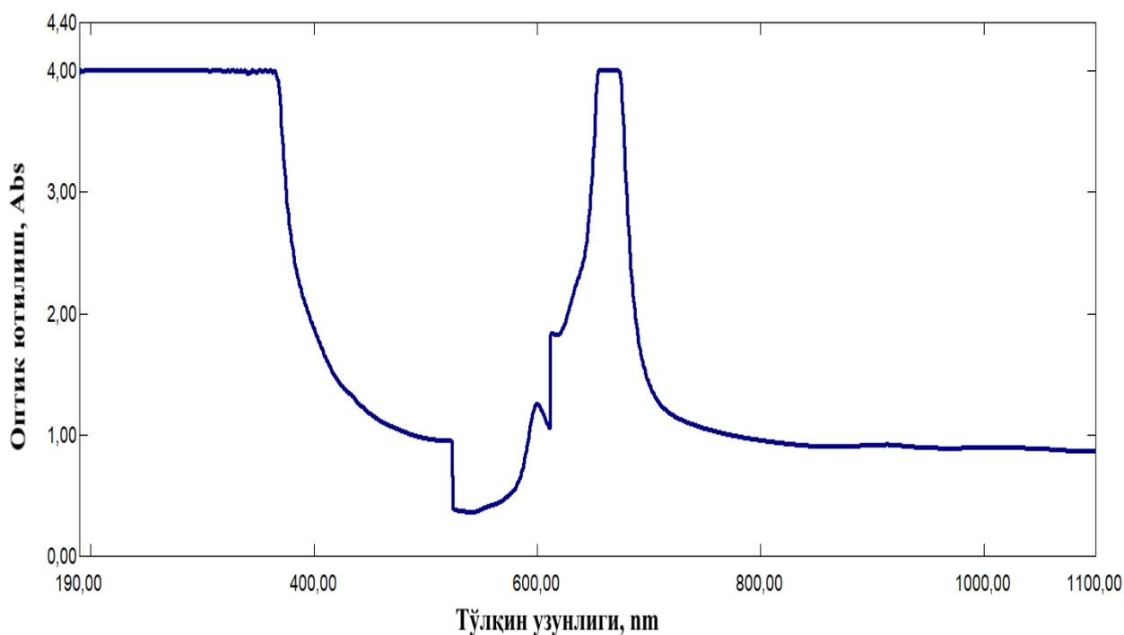
**Figure 2.14. Ratio of light absorption to wavelength of K-1 brand organic pigment**
