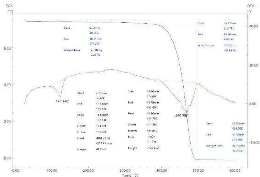
**Figure 3.21. Thermogravimetric derivatogram of polyethylene brand 0320.**
