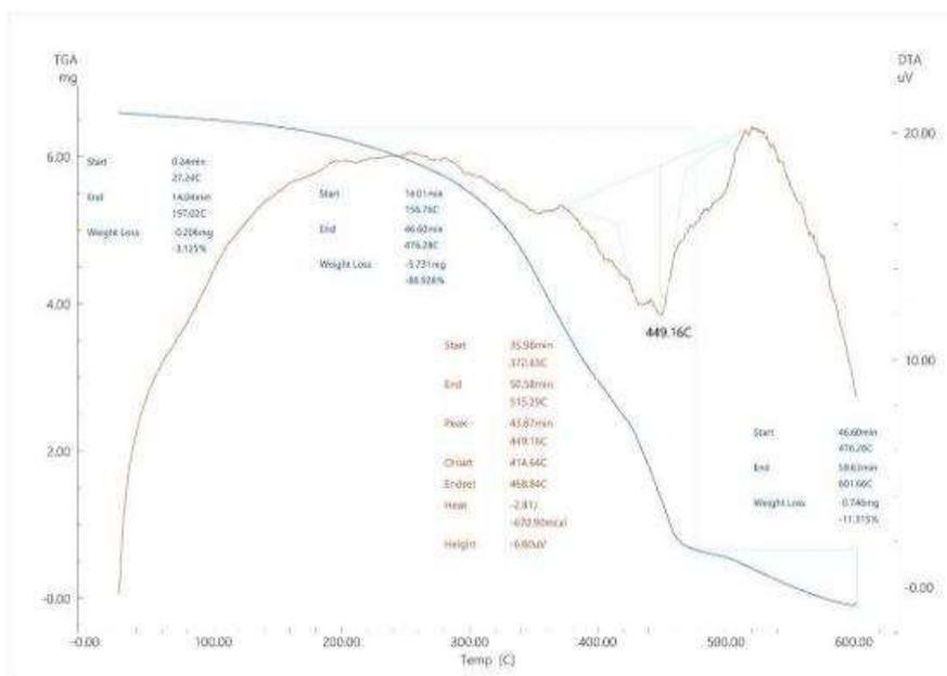
**Figure 3.4. Derivatogram of alkyd enamel made on the basis of K-1 organic pigment**
