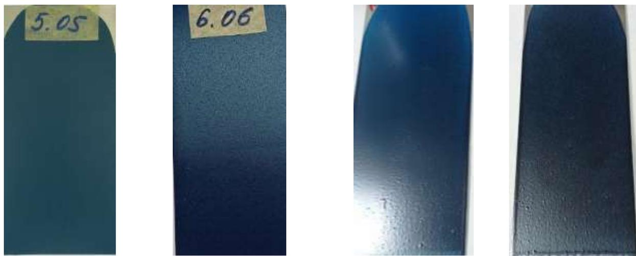
**Figure 3.1. Alkyd enamel coated on a metal plate (based on new pigments).**
