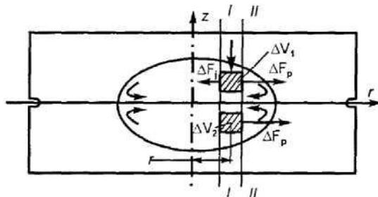
**Figure 3.** Distribution of forces acting on particles suspended in a solution
