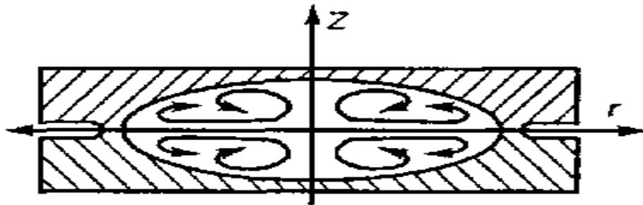
**Figure 1.** Direction of rotation of the liquid metal core during mixing. It is this current that causes the liquid metal to mix with the welding current.
