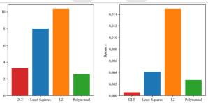
For the selected triangulation methods, a series of experimental tests were also carried out, during which, for each approach, the calculated lengths of the user's limbs and the absolute deviation of the obtained values from the real ones were measured. The comparison is presented in Table 1.
