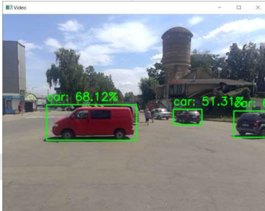
Figure 1: The developed user interface of the object identification program based on the MobileNetV2 neural network for a mobile robot
