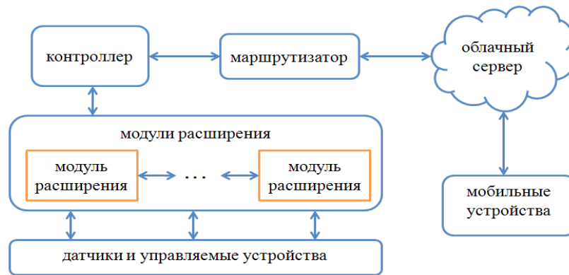
Rice. 2. Scheme of technical support for an intelligent industrial building with remote control function via the Internet
