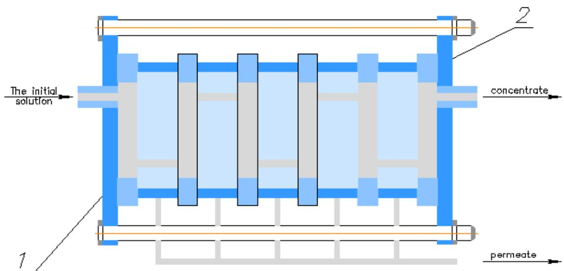
*Fig. 1. A flat-chamber multi-section apparatus of the "filter press" type (1 — membrane; 2 — drainage material )*
